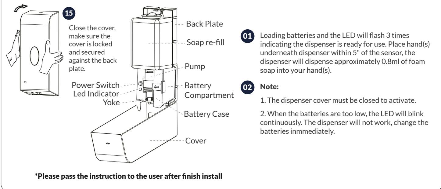
**15** Close the cover, make sure the cover is locked and secured against the back plate.
