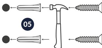
5. Place the plastic anchors in the holes and push them with the help of the hammer.
